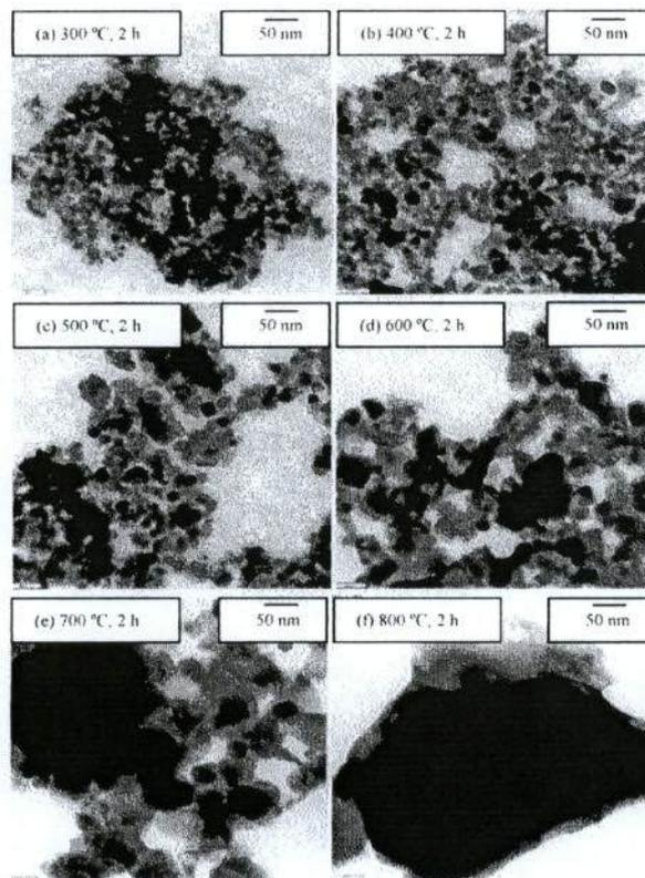
Fig. 4. TEM images of as-synthesized nanosheets TiO<sub>2</sub> calcined at various temperatures for 2 h at (a) 300 °C, (b) 400 °C, (c) 500 °C, (d) 600 °C, (e) 700 °C and (f) 800 °C.
