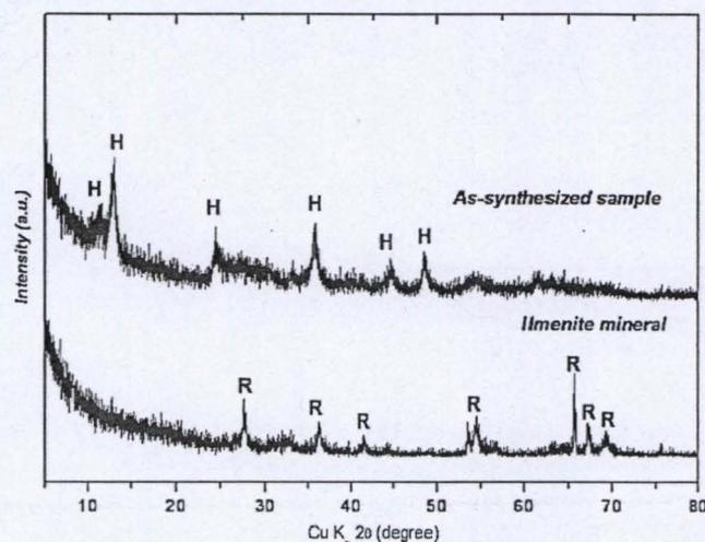
Fig. 3. XRD patterns of the starting ilmenite mineral and the as-synthesized sample, H=hydrogen titanate and R=rutile TiO<sub>2</sub>.
