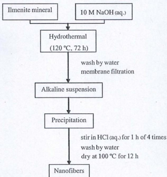
Fig. 1. Schematic representation of the experimental procedure.
