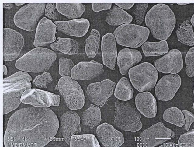
Fig. 4. SEM image of the starting ilmenite mineral.
