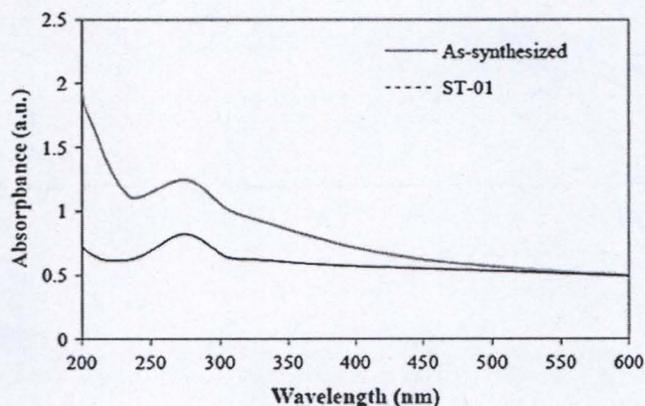
Fig. 8. UV-vis absorbance spectra of the as-synthesized nanofibers and commercial grade TiO<sub>2</sub> nanoparticles (ST-01).
