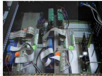
Fig. 5 Motor drive compartment for joint 4, 5, 6.
