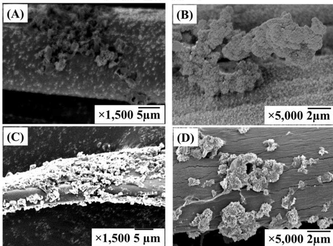
**Figure 2** SEM images of calcium phosphate and hydroxyapatite crystals on various soaked time (A, B) silk fibers soaked in SBF for 7 days and (C, D) silk fibers soaked in SBF for 30 days
