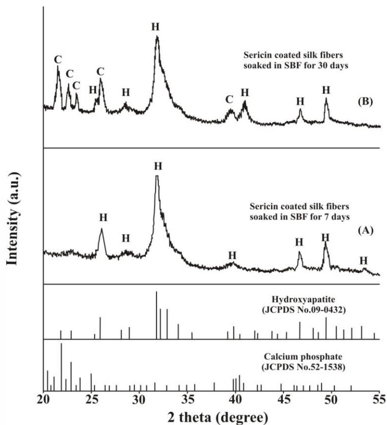
**Figure 1** XRD patterns of HAp and calcium phosphate crystals on silk fibers after soaked in SBF at 7 days and 30 days
