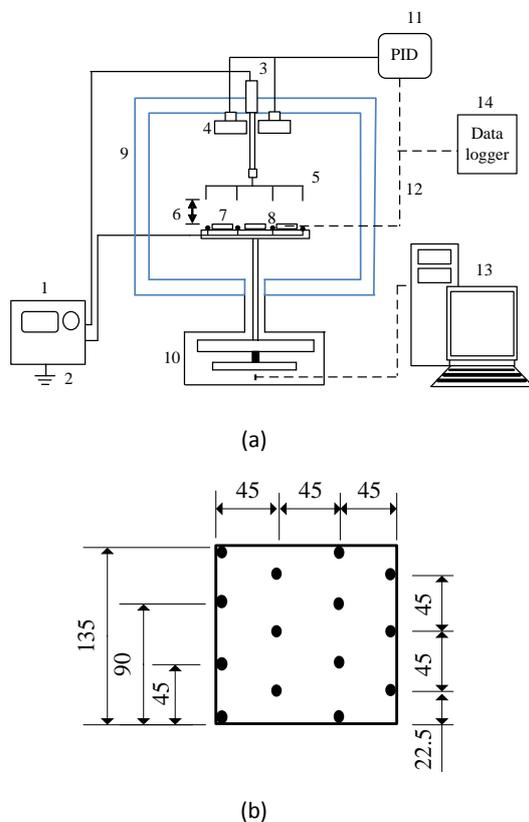
Fig. 1 a) Schematic diagram of EHD-FIR drying system in side view; 1 high voltage power , 2 ground, 3 adjust probe, 4 far – infrared radiator, 5 anode electrode, 6 electrode gap, 7 samples, 8 cathode electrode 9 drying chamber, 10 load cell, 11 PID controller, 12 thermocouple, 13 computer, 14 data logger
