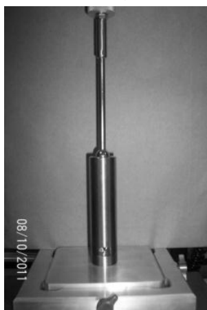
Fig. 2 Back Extrusion test platform
