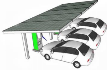
Fig.2. The example of solar-powered charging station for electric vehicle.
