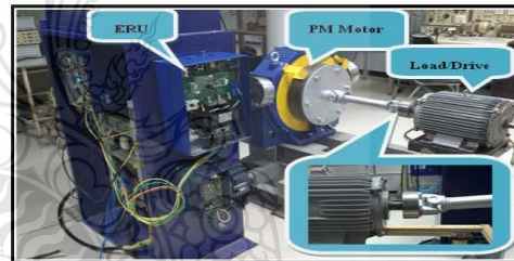
Fig 6, Energy Regenerative (EERU) Laboratory Prototype
