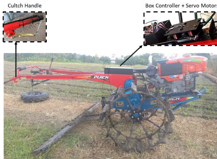
Figure 4.40. Quick G1000 Tractor Box Controller Installation
